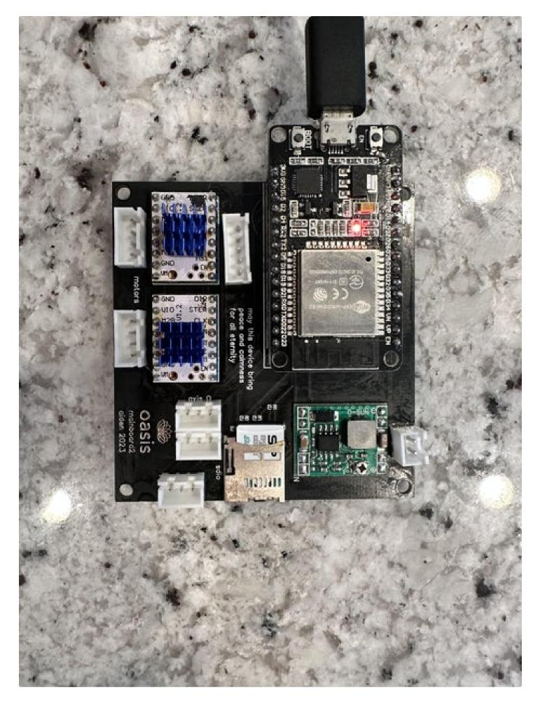
ESP32-Powered Tabletop Kinetic Sand Drawing Robot: Page 16
